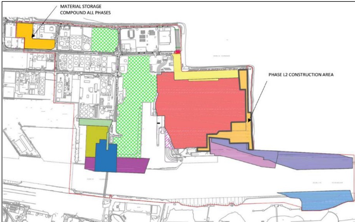
Figure 3-26 Phase L2 Construction Area
